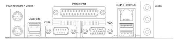
Figure 1-3. Back Panel Connectors
